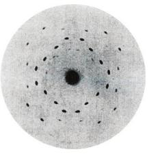
Max von Laue discovered that X-rays beamed through a crystal onto a photographic plate acquire a clear diffraction pattern.
